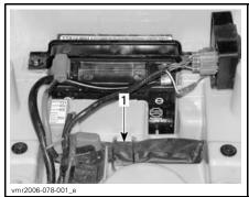
SERVICE COMPARTMENT UNDERNEATH SEAT 1. Tool kit
